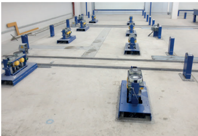
High-frequency compactors equipped with magnets in a MagVib compaction station.
