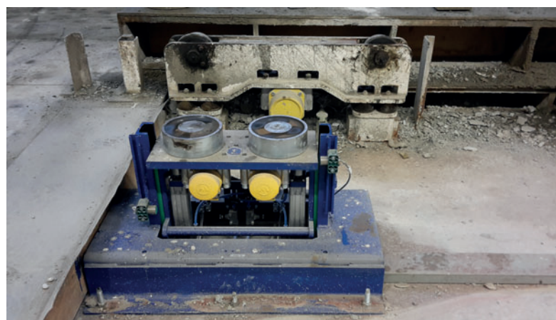
MagVib high-frequency vibration unit (blue), the vibrating trestle used previously is in the background.
