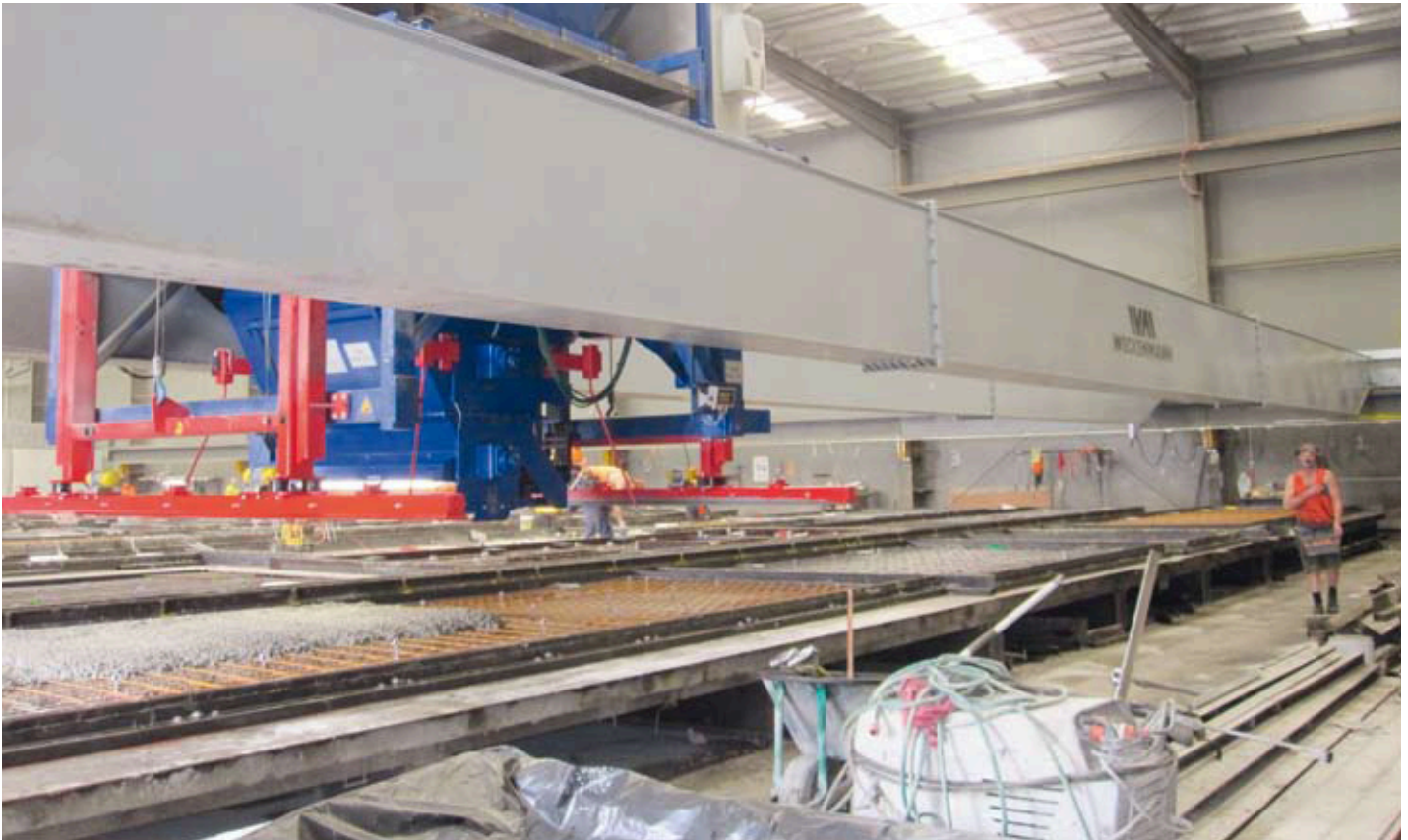
Fig. 2 The new concrete distributor from Weckenmann in use during the concreting process. Manually operated with radio remote control.
