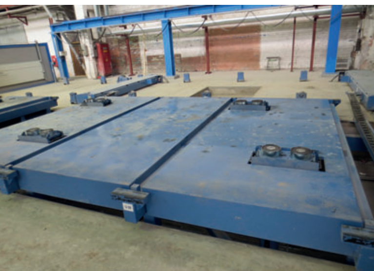
Combined shaking/vibrating station with high-performance electromagnets
