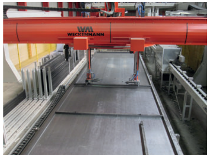
Le robot Weckenmann Twin-Z hautes performances
