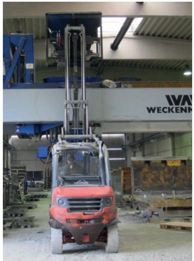
The bucket of the concrete distributor is still filled by fork-lift truck; in the near future the concrete will be filled directly into the concrete distributor via a branch line from the new mixing plant, which is currently being planned.
