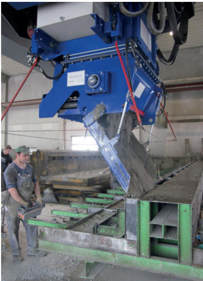
All mould heights can now be driven to flexibly and with the utmost accuracy by just one operator with the new concrete distributor.
